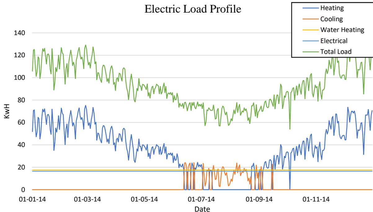
**Figure 1.** Grid Load Profile Over 2014 for an Average House in PEI
