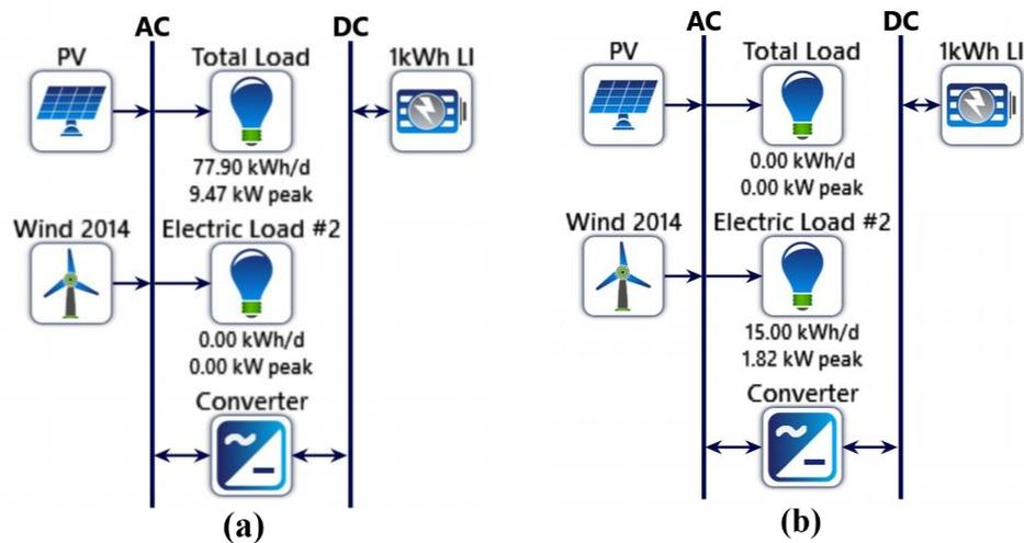
**Figure 2.** (a) Schematic Diagram of HOMER Simulation for Full House Load
