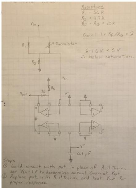
Figure 3: Thermistor linearization circuit with amplifier
