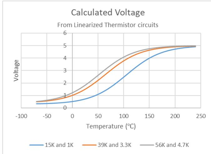
Figure 12: Voltage curves calculated using Equation 9
