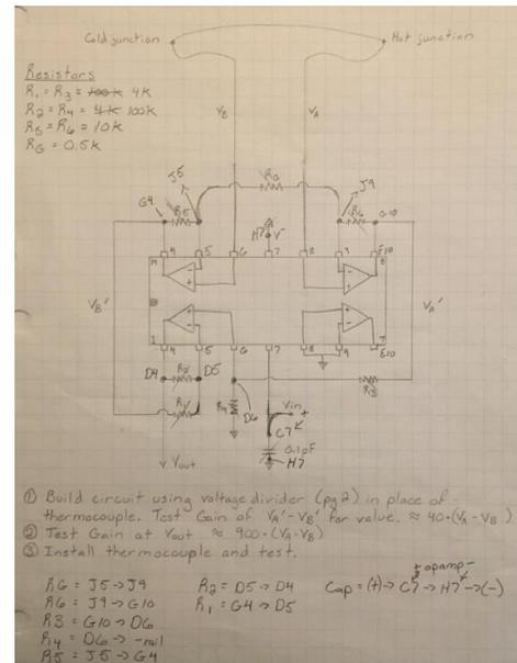
Figure 7: Thermocouple circuit with nodes labeled for prototyping board
