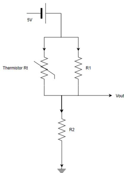
Figure 1: Thermistor linearization circuit set up on a bread board to measure the voltage for different temperatures and values of R1 and R2.
