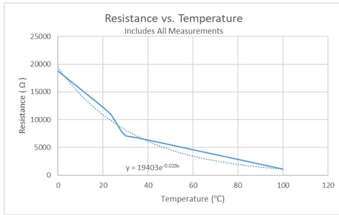
Figure 8: Resistance vs. temperature curve plotted from Table 1
