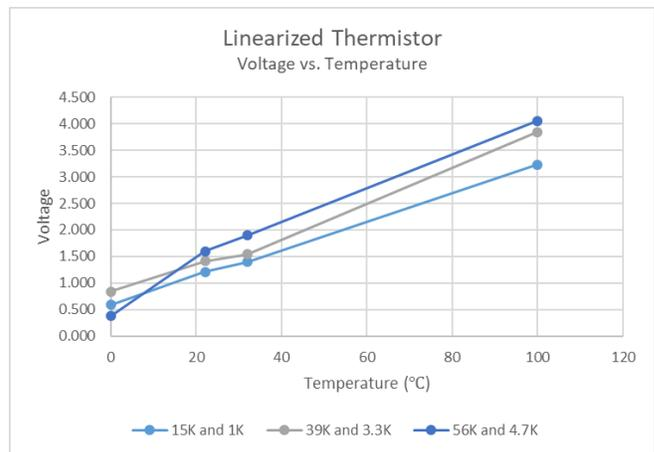
Figure 11: Output voltage from the linearized thermistor circuit for different temperatures
