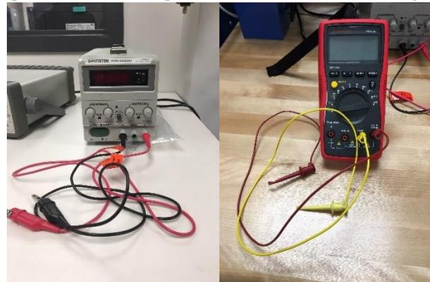
Once we thought we had the instrumentation amplifier working we attempted to test it using the provided thermocouples.
