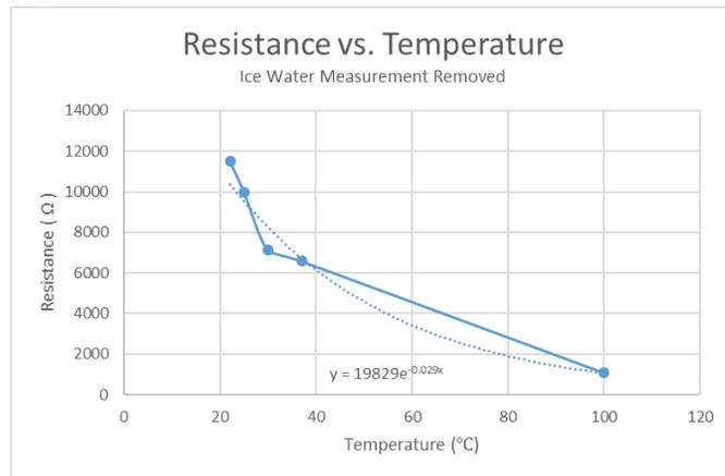
Figure 9: Resistance vs. temperature curve plotted from Table 1 with 0°C measurement removed
