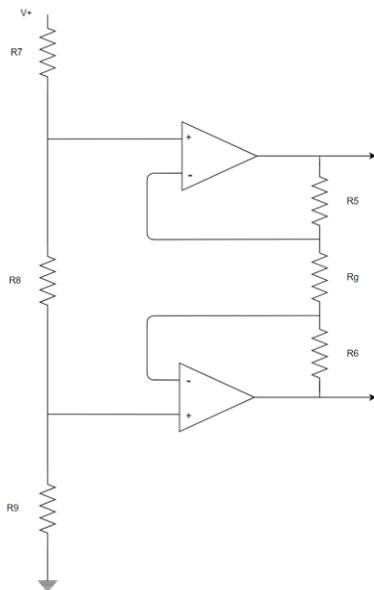
Figure 4: First stage of instrumentation amplifier
