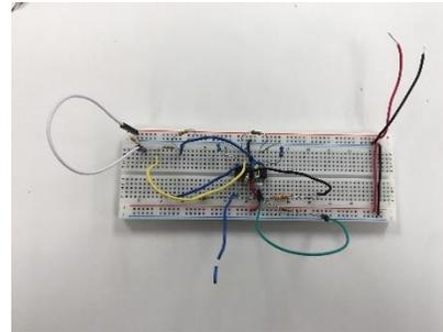
We used a LM358AN op-amp to amplify the output from the thermistor linearization circuit and were to use the LM324AN op-amp to create the instrumentation amplifier to amplify the thermocouple's output. We used the labs power supply and Amprobe multimeter to power the circuit and take readings.
