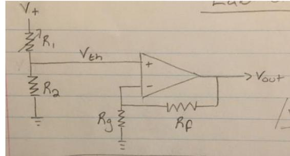
Figure 2: Operational Amplifier, non-inverting gain circuit
