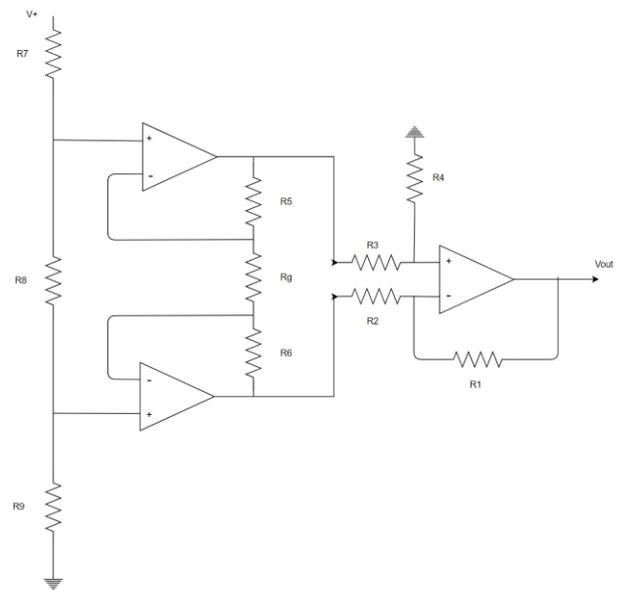
Figure 5: Instrumentation amplifier, stage one and two
