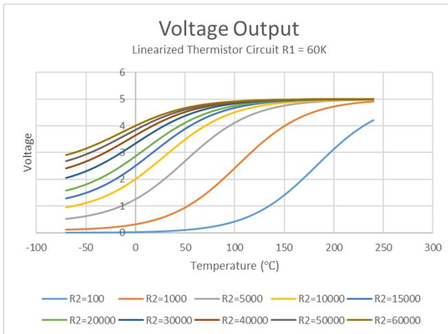
Figure 13: Voltage curves calculated using for a fixed value of  $R1$  using Equation 9
