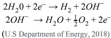
The polymer membrane of a Polymer Electrode Membrane (PEM) Electrolyzer prevents gaseous  $H_2$  and  $O_2$  from passing through but allows  $OH^-$  ions to pass through. There are multiple different types of electrolyzers, all with different efficiencies, but this method is the most environmentally friendly and has an efficiency from 80% to 60%. Currently, this accounts for about 4% of global hydrogen production. As technology improves, so will electrolysis efficiency.
