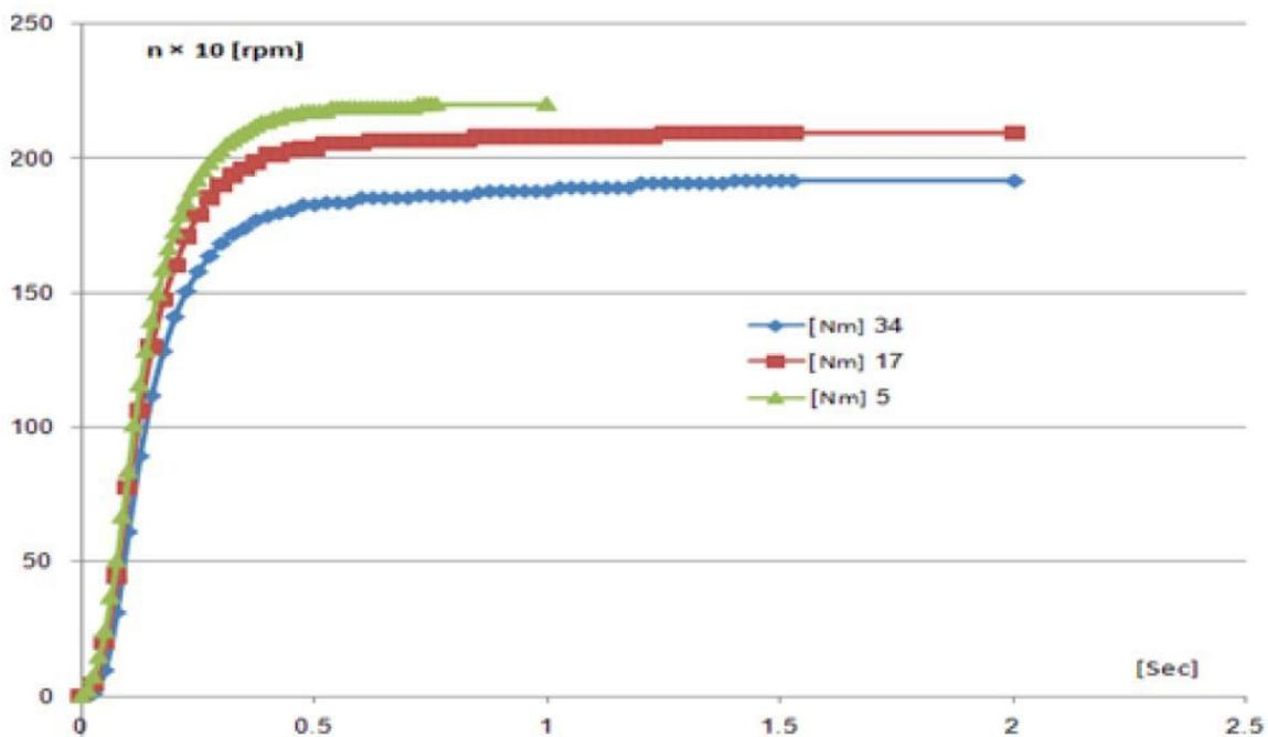
Figure 4 shows consistent results over different loads the ability to accelerate to a constant rpm. This makes the inverter motor a much more viable option in electric cars instead of heavy permanent magnet motors, allowing for a lightweight motor to be installed into electric cars.
