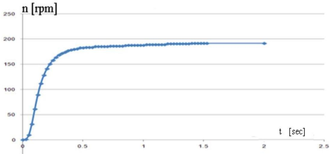
Figure 4 shows the rotation speed of an inverter motor when 34.4 Newton meters are applied. Y axis shows rotation speed in revolutions per minute, and the x axis shows time (Bitar, 2012). The steep acceleration curve shows that the rpms level out consistently, giving the motor a steady rotation speed.
